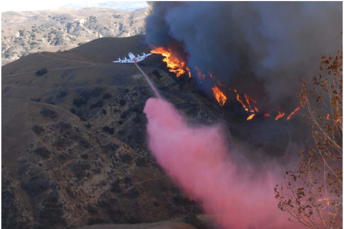
Air tanker lays a retardant line in front of the fire to slow its forward progress.
