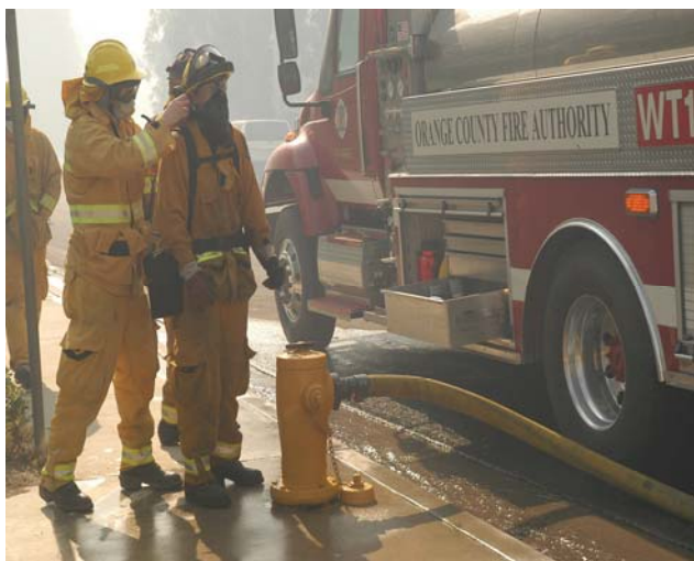
Firefighters fill a Water Tender at a lower elevation to take to engines fighting fires at higher elevations due to the lack of hydrant pressure.
